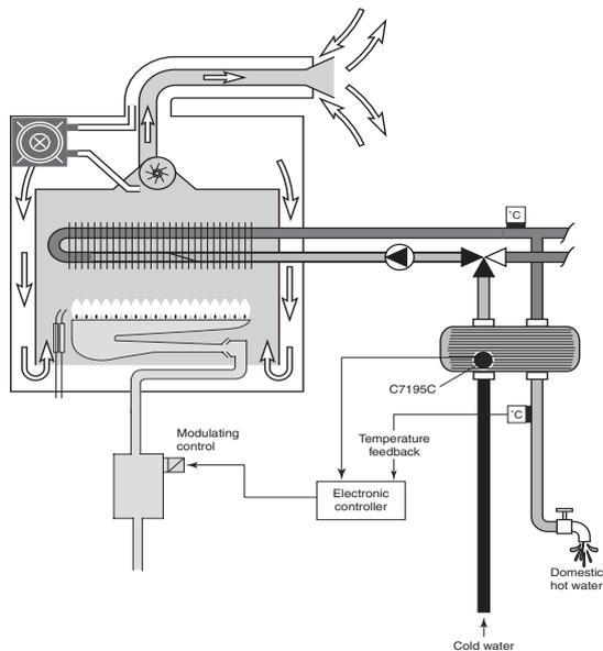
**Fig. 2. Instantaneous combi boiler with feed forward or feedback control loop**
