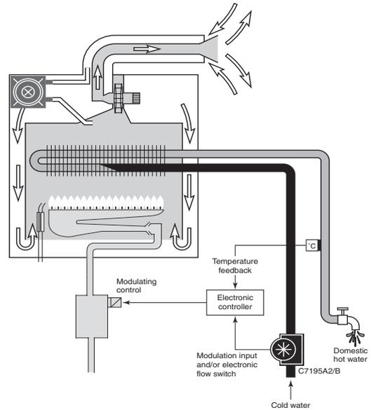
**Fig. 3. Instantaneous water heater with feed forward or feedback control loop**
