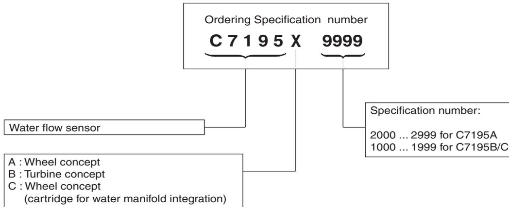
Fig. 12. Model number chart C7195A/B/C water flow sensor
